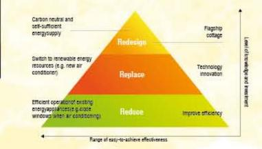
The engaged 3R methodology provides a progressive approach. It starts with simple measures that are easy to implement, but remarkably improve energy performance (Reduce). The next step is to invest the savings from the previous Reduce solutions in substituting fossil-based and outdated technologies with more efficient and greener ones (Replace), followed by a total redesign of resort establishments providing a Zero Carbon system for future energy services (Redesign).
